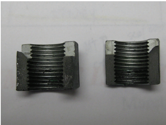
Photo Photos of first nut before removal (above) (still safetied); and after its removal (below) when it broke in half as it was removed.
